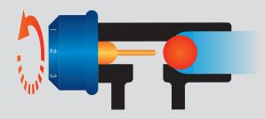
To turn off, return to original OFF position. A partial turn to the OFF position will minimise the volume of water when in use.
