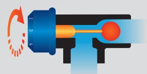
**Easily** rotate towards ON for a gradual increase in water pressure. A partial turn will minimise the volume of water when in use.
