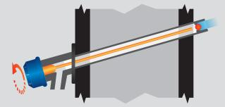
To turn off, return to original OFF position. A partial turn to the OFF position will minimise the volume of water when in use. The angle of the tap will drain the excess water, stopping the bibb from freezing in winter!
