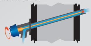
**Easily** rotate towards ON for a gradual increase in water pressure. A partial turn will minimise the volume of water when in use.
