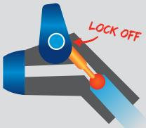
To turn off, press the Lock button back to the original position. The water pressure will automatically turn the spray off!
