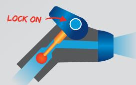
To turn on, simply pull the lever towards yourself! Lock it ON by pressing the lock button. Minimal effort is required!
