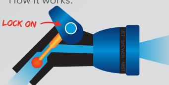
To turn on, simply pull the lever towards yourself! Lock it ON by pressing the lock button. Minimal effort is required!
